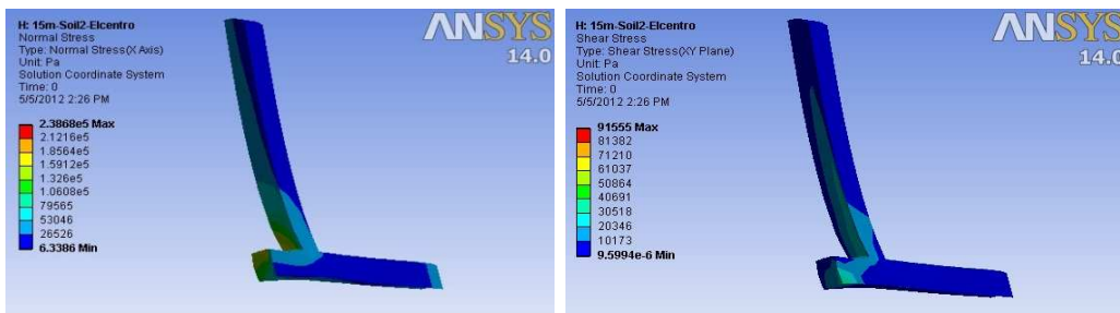
Fig11. Normal and Shear Stress of wall for Soil 2 under El Centro Earthquake
