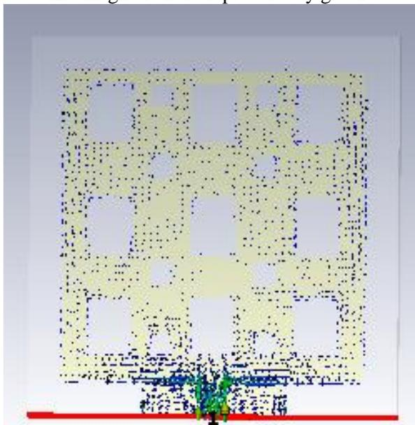
Figure 9: Surface current of proposed antenna
