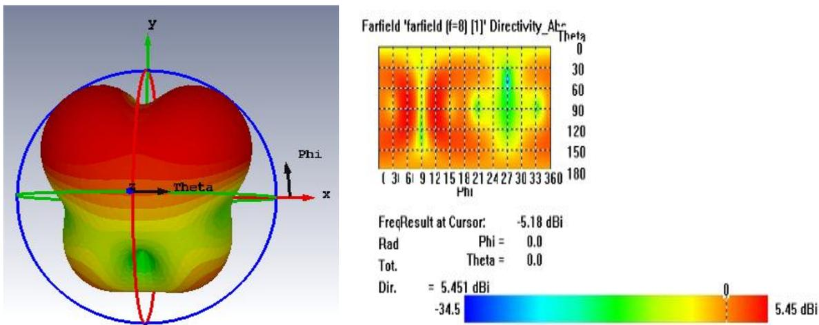
Figure 8: 3D Radiation pattern and Directivity 2D plot of proposed antenna band
