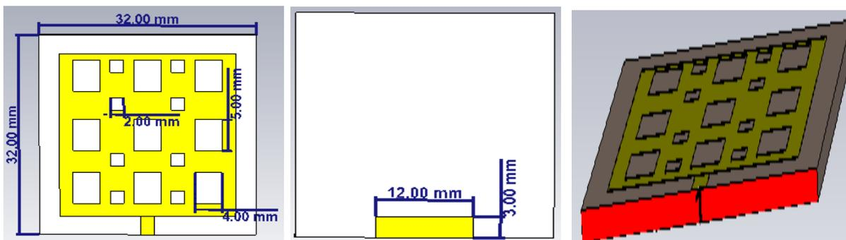
**Figure 2: Dimension of proposed antenna and Side view in CST Studio**
