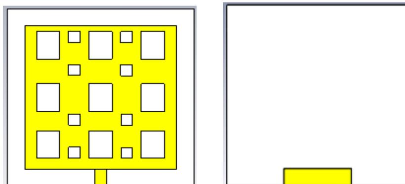
**Figure 1: Top view and Bottom view of proposed antenna**
