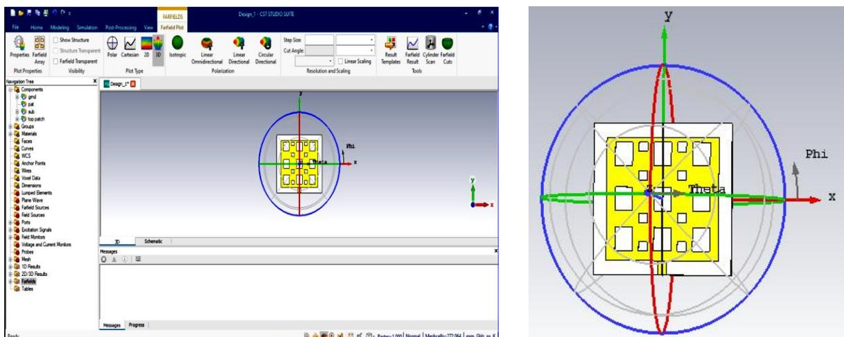
**Figure 3: CST view of proposed antenna**
