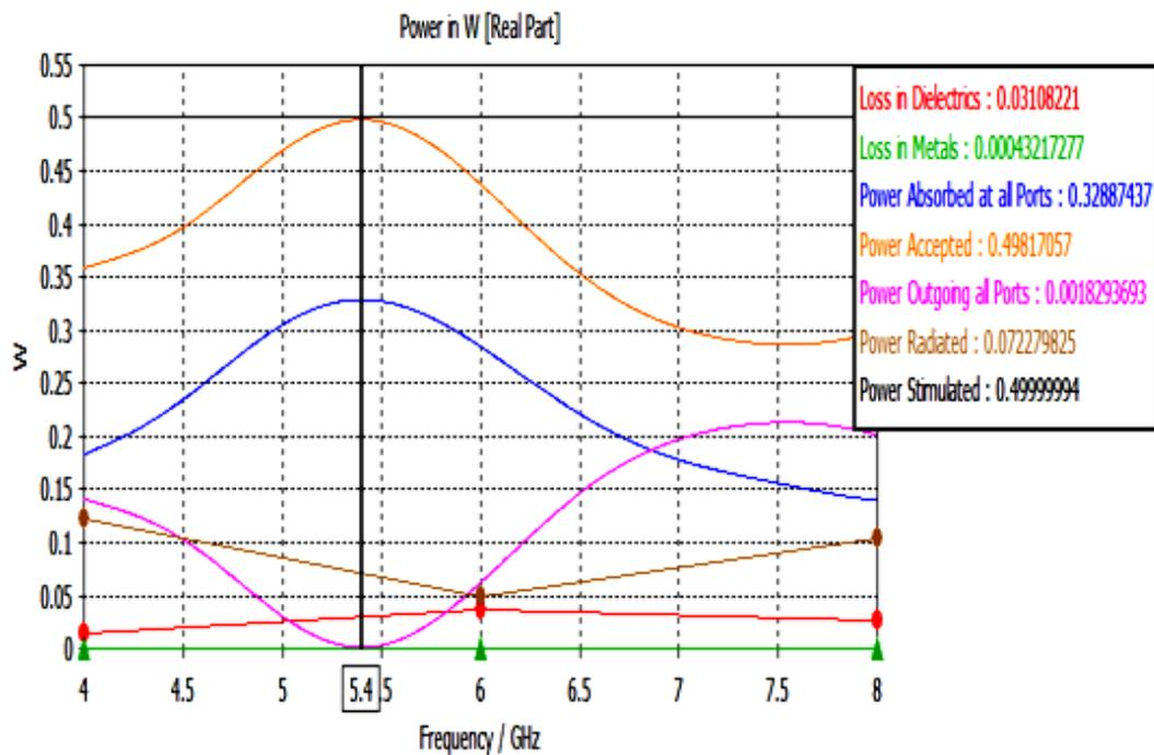
Figure 7: Power in different port for first band
