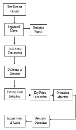
The SIFT descriptor is based on image in terms of fields and frames. This defection and description of local images features can help in object recognition. They are relatively easy to match against a large database of local features, however the high dimensionality can be issue and generally probabilistic algorithm.
