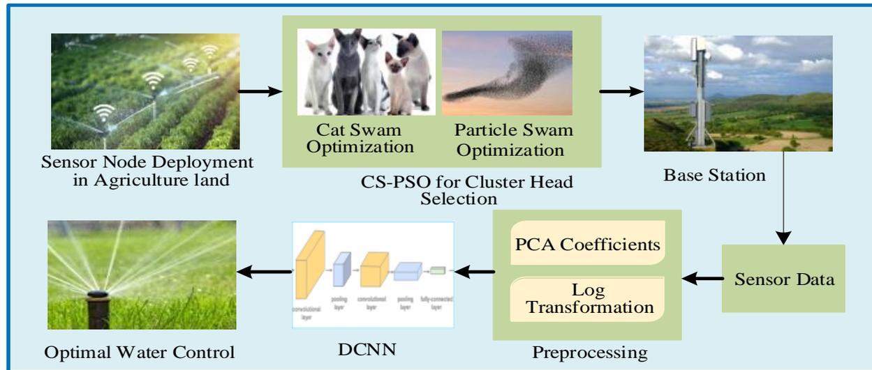
**Figure 1:** Architecture of proposed CS-PS optimization based Deep CNN for optimal water control
