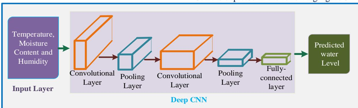
Figure 3: Deep CNN Architecture
