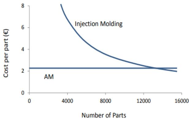
**Fig 1: Cost Model Compared to Injection Molding [7]**
