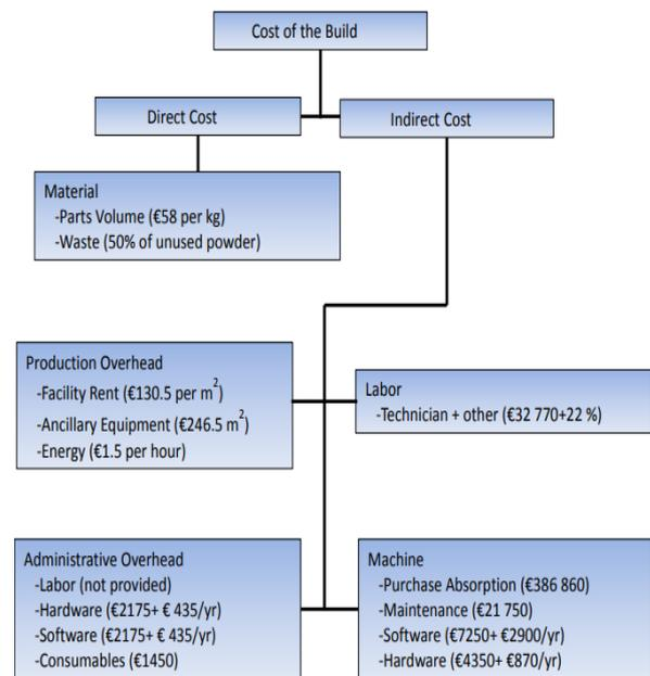
**Fig 2: Cost Model for Additive Manufacturing [8]**
