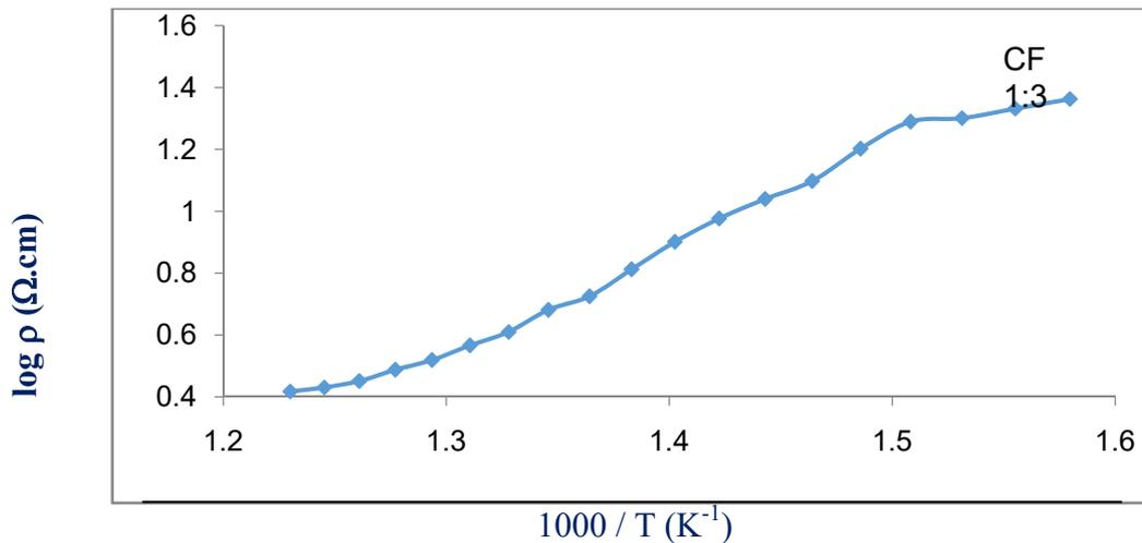
Fig.3: d.c. electrical resistivity
