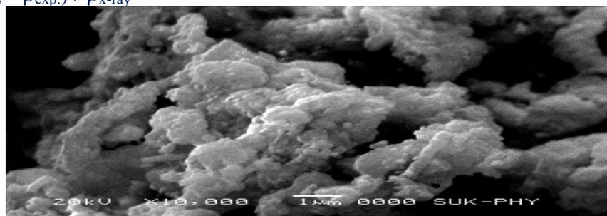
Fig. 2: SEM image of copper ferrite
