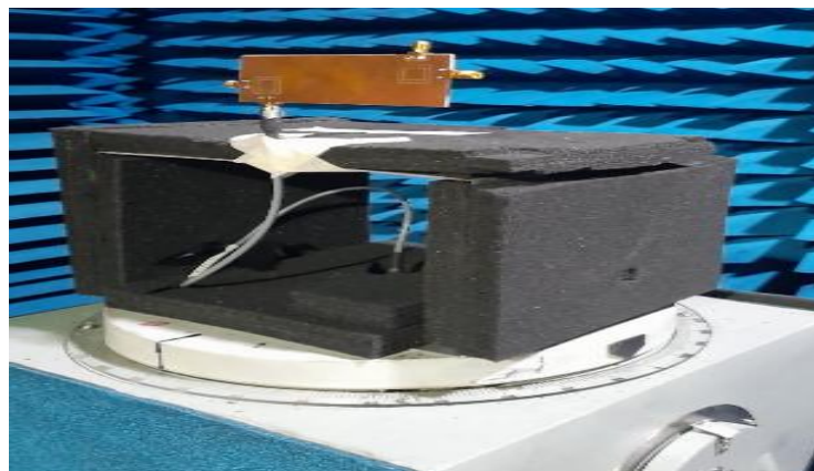
Figure 5: Proposed Antenna in Anechoic Chamber
