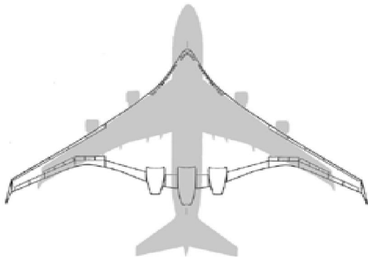
Fig.1(b):Blended wing body structure vs conventional structure ( The Blended Wing Body Concept , n.d.)
