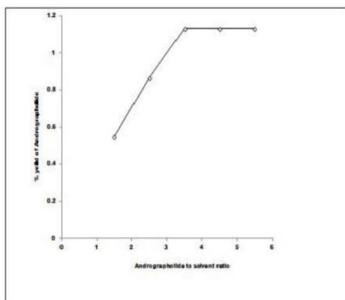
Figure 3: Effect of dry feed to solvent ratio on the percent yield of andrographolide
