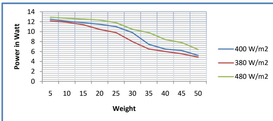
Figure 9. Power-to-weight relation for dune sand
