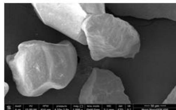
SEM image for the dune sand (50 μm and 100 μm)
