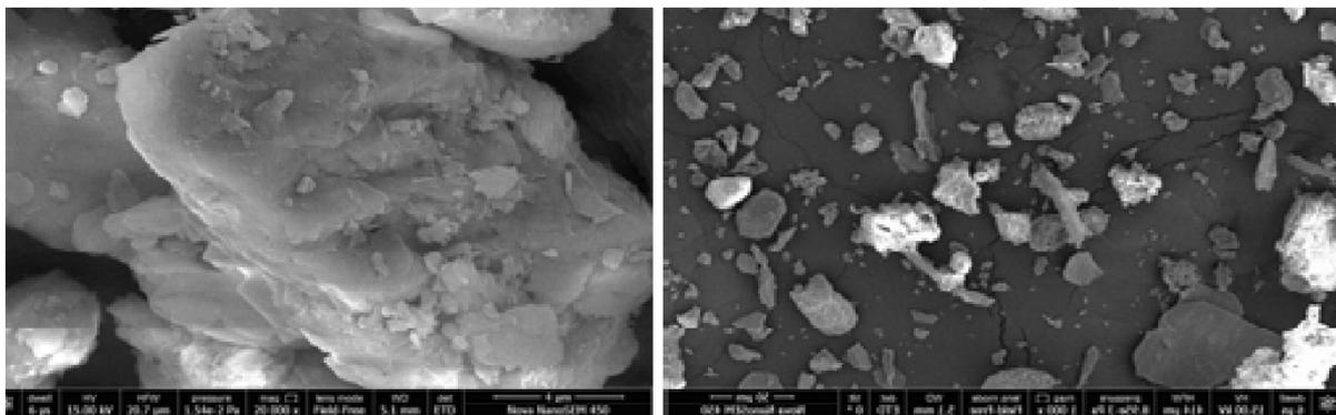
SEM image for dust collected from solar panel (4 μm and 10 μm)
