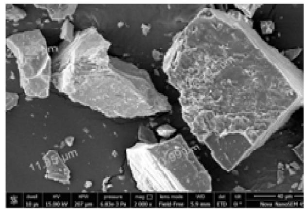
SEM image for the marble dust (10 μm and 40 μm)
