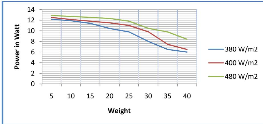
Figure 7. Power-to-weight relation for dust collected from panel
