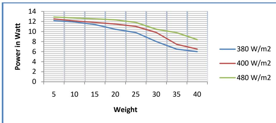
Figure 8. Power-to-weight relation for marble dust
