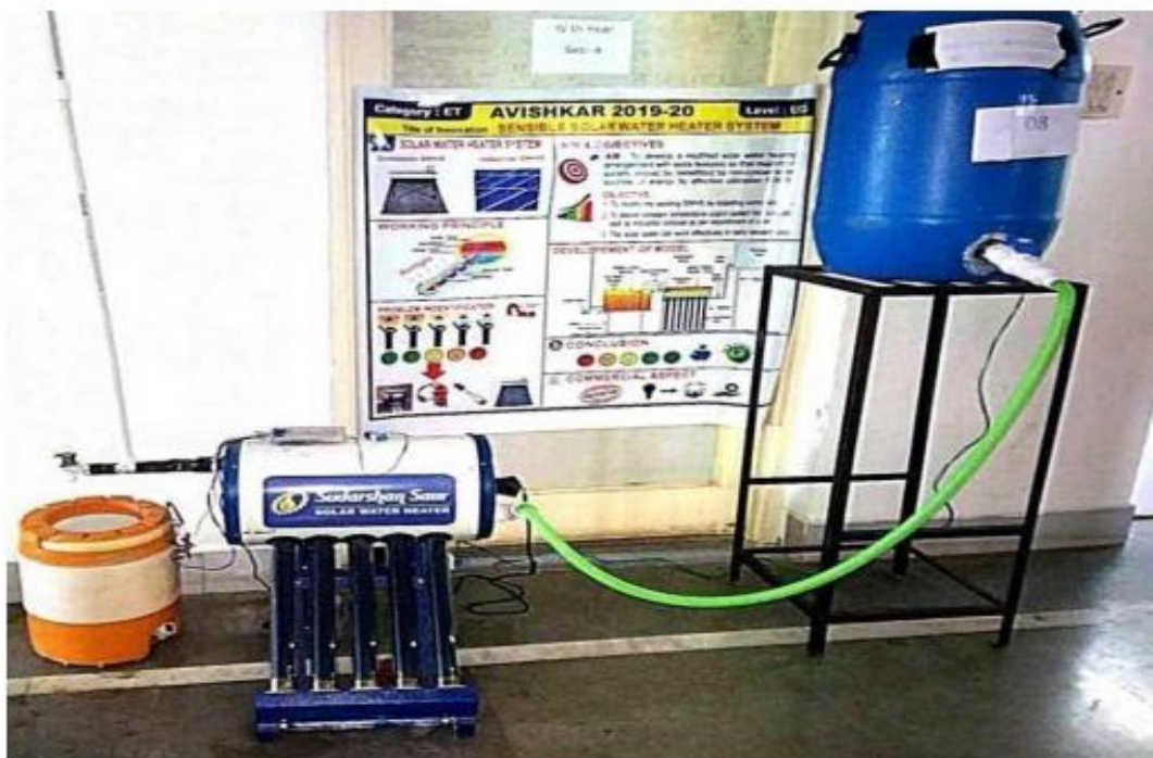
Fig.2 : Prototype of modified solar water heating system
