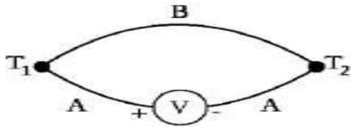
Thermoelectricity means the direct conversion of heat into electric energy, or vice versa. According to Joule's law, a conductor carrying a current generates heat at a rate proportional to the product of the resistance (R) of the conductor and the square of the current (I). A circuit of this type is called a thermocouple.
