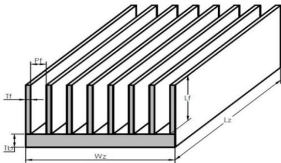
Fig.7- Rectangular Heat Exchanger Geometry
