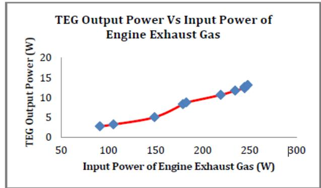
Fig.8-TEG Output Power Vs Input Power
