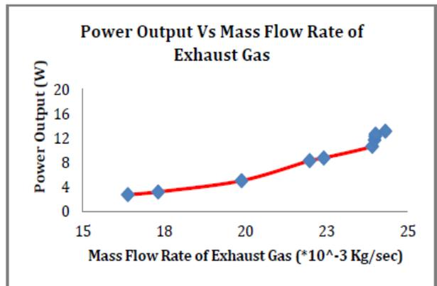
Fig.9- Power Output Vs Mass Flow Rate of Exhaust heat Gas
