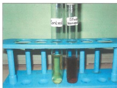
Photo plate 2 : Synthesis of Silver nanoparticles by Mentha piperita extract
