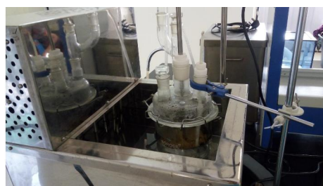
[Fig 1 : Assembly for making Soya adhesives]
