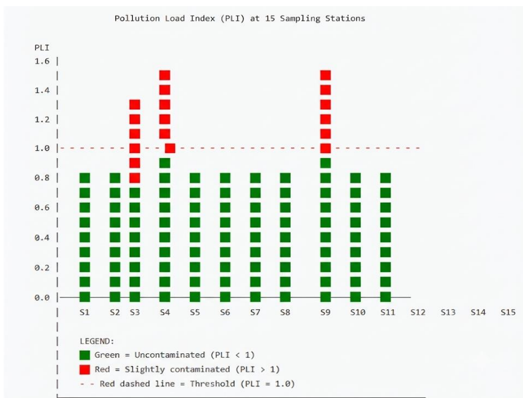
Figure 1. Pollution Load Index (PLI) at 15 sampling stations in the Mahad MIDC area. The horizontal dashed line at PLI = 1.0 represents the threshold for soil quality deterioration.
