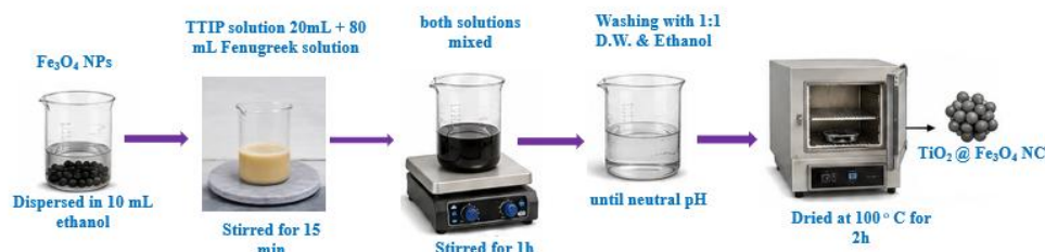
Fig.1: Schematic illustration of the stepwise synthesis of \text{Fe}_3\text{O}_4 nanoparticles and \text{TiO}_2@\text{Fe}_3\text{O}_4 nanocomposites.
