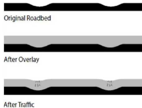
Figure 2. Overlying over Distressed Asphalt Pavement
