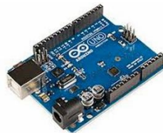
Fig. 2. Arduino Uno: Microcontroller for processing sensor data and controlling outputs
