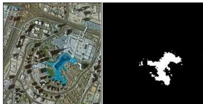
Fig. 2. Input satellite image & system output for Waterbodies detection
