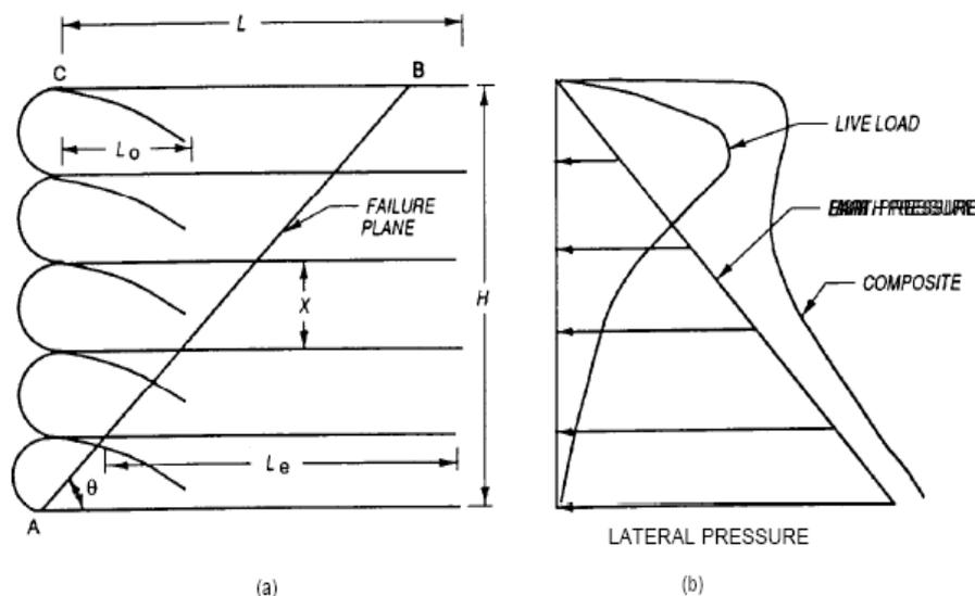
**Fig. 1** General Configuration of a Geotextile Retained Soil Wall and Typical Pressure Diagrams
