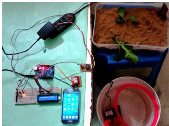
Figure 10 A Designed Prototype of Automatic Irrigation System Using Soil Moisture Sensor
