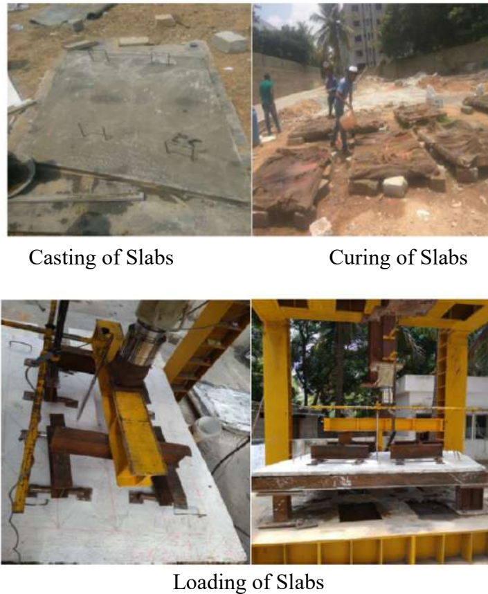
Figure 2 Experimental Working Stages of Skew Slabs
