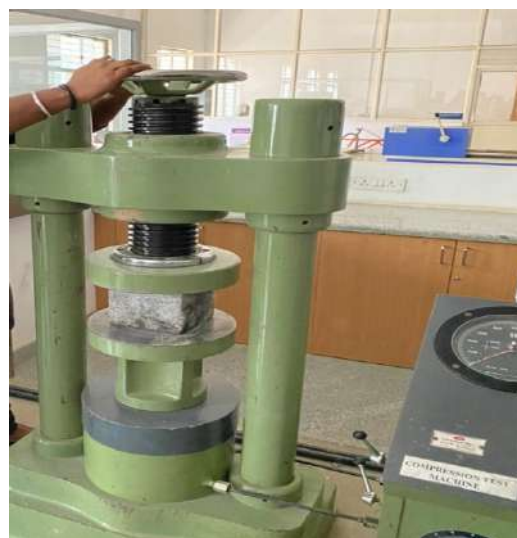
Figure 1: Compressive Testing Machine
