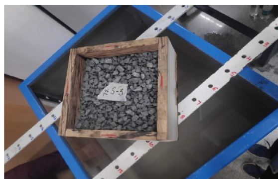
Figure 7: Permeability test on No-Fine Concrete slab
