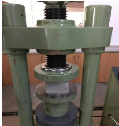
Figure 7: Compression Testing of Cube in CTM
