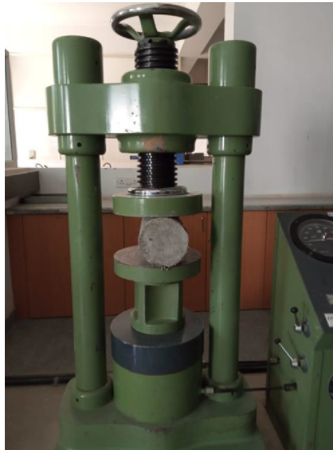
Figure 9: Split Tensile Testing of Cylinder in CTM.
