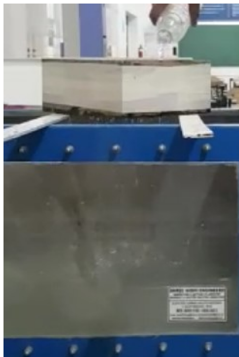
Figure 2: Water passing through the permeable concrete slab
